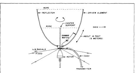
fig. 3. The K2GNC "rotary ground plane." This interesting vertically polarized array consists of a 1/4-wave driven element and reflector working against four 1/4-wave radial ground wires. The driven element is fed with a gamma match. All elements are connected to the tower (or mast) at center point, as are the radial wires.
